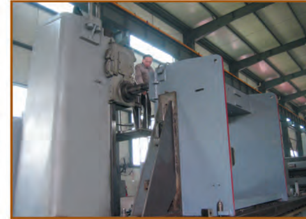
30 Ft G&L Horizontal Boring Mill provides greater capability for machining of large welded and stress-relieved structure ensuring highest degree of accuracy
