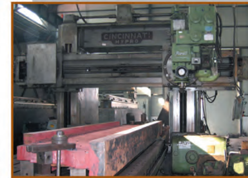
30 Ft G&L Horizontal Boring Mill provides greater capability for machining of large welded and stress-relieved structure ensuring highest degree of accuracy
