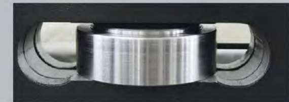
Hydraulic CNC auto Crowning System Crowning cylinder mounted in bed and provides automatic anti-deflection compensation correlated to tonnage
