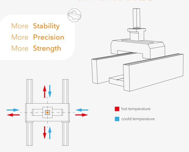
The expansion of hot or coold temperature does not interfere with the center, so this system can be ensured to have the execellent precision during machining.
