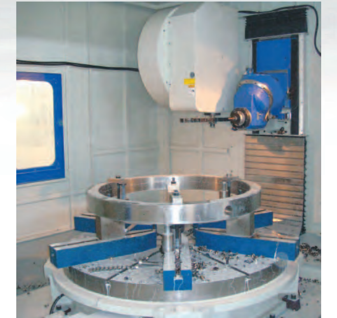
• Standard automatic vertical & horizontal milling head with BT#50/3500RPM/811Nm
