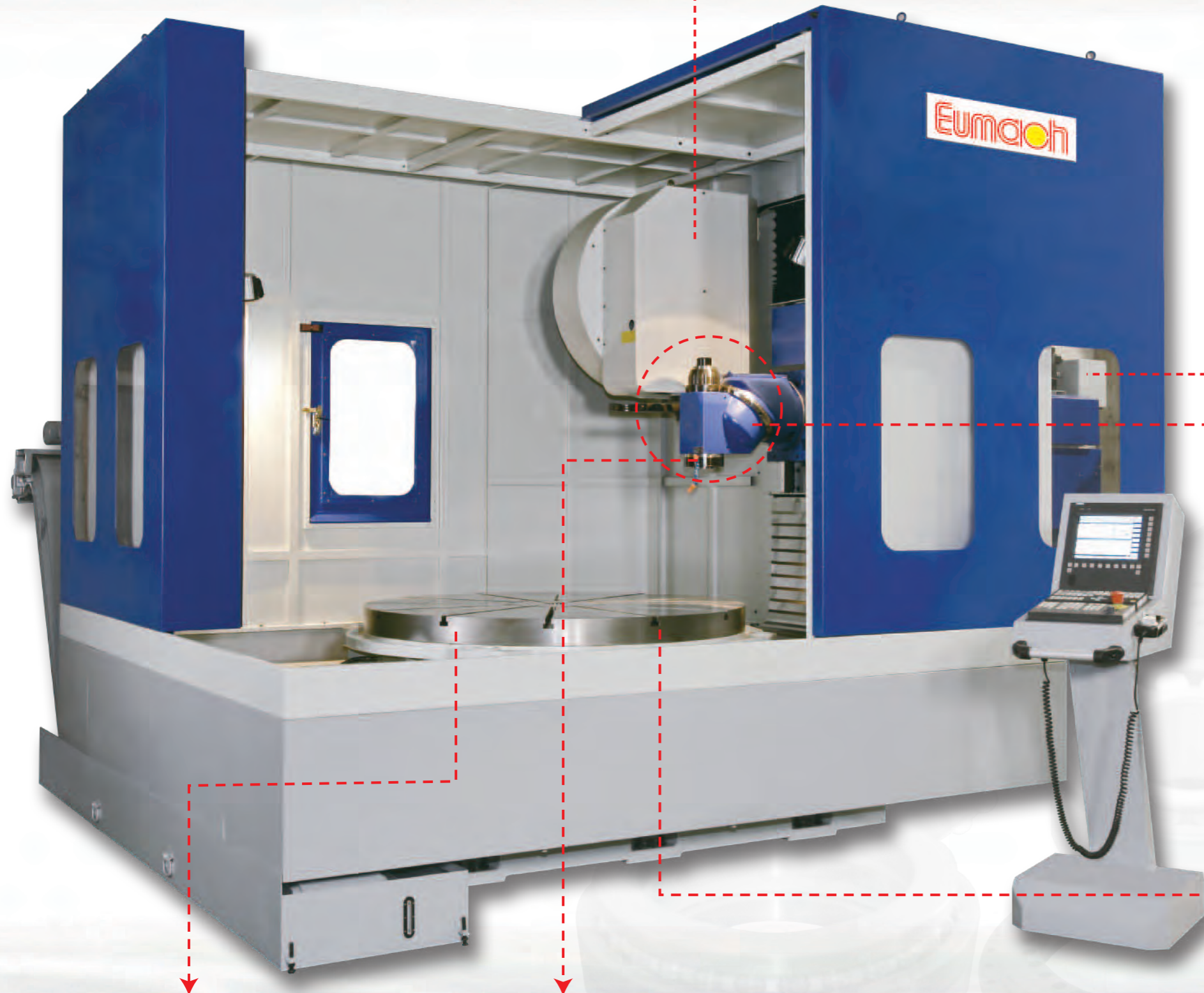
• Standard \phi 1650mm CNC rotary table, 8000kg load.
