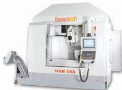
◦ HSM-5X 1020 / 610 / 810MM, BT#40, 14000RPM
