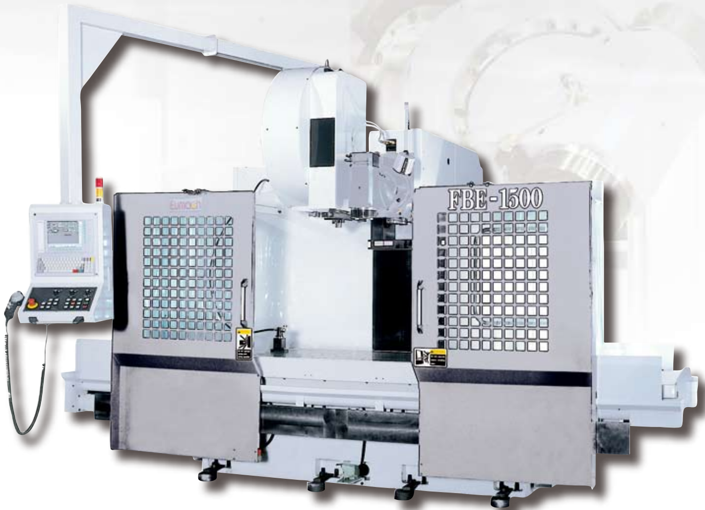
► FBE-1500 with 1500mmx1000mmx950mm(1500mm) travel, 1600mmx1050mm table
