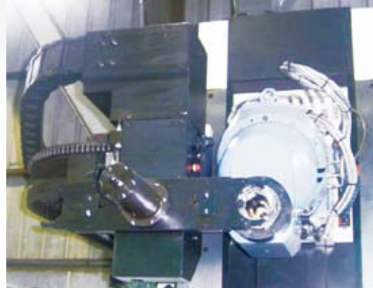
Horizontal tool change with 32, 40 or 60 stations swing arm rail type
